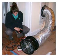
common performance tests are associated with building envelope tightness (blower door test), and when mechanical system ductwork resides outside the building thermal envelope, duct tightness (duct blaster test).
