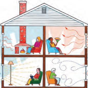
**U-factor** measures the heat from **INSIDE** a room that can escape. The lower the number the lower the potential for wasted heating expenses.
